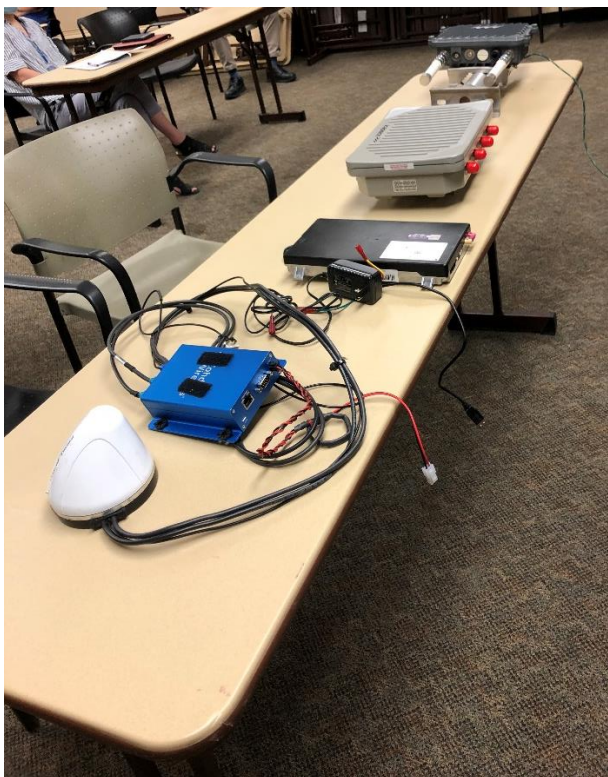
Examples of CV equipment and antennae to be installed on vehicles and at intersections.
